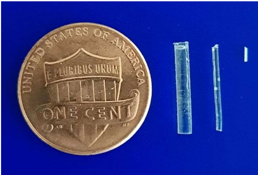
Figure 1: Injection molded PEA rods with diameters of 2000, 850, and 200 \mu\text{m} (L to R).
